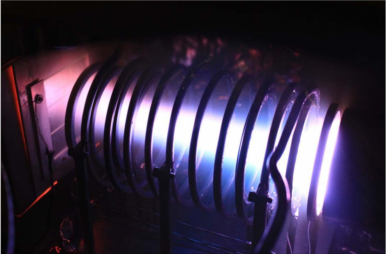
Fig. 1. Plasma lens placed between (right) magnetron and (left) substrate. The magnetron has a 2-in (5 cm) diameter aluminum-doped zinc target, operating in an argon–oxygen gas mixture. Microscope slide substrates are mounted on a heater; the goal is to deposit high-quality AZO films, a low-cost transparent conductor.
