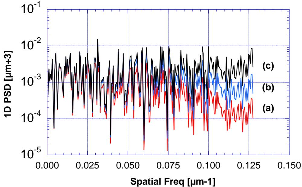
Figure 7: 1D PSD spectrum of the prototype BPRG with 4095 total number of elements with 2.5- $\mu\text{m}$  pitch measured with the Micromap<sup>TM</sup>-570 microscope with 2.5x objective: a) (lower, red) average uncorrected raw PSD curve; b) (middle, blue) corrected to account for MTF due to the objective lens aperture, and c) additionally corrected for the MTF of the finite pixel width.
