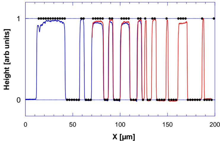
Figure 2: Measured profiles made near the left edge of a prototype BPR grating with a Micromap<sup>TM</sup>-570 interferometric microscope with a 50x objective. Also shown are the corresponding points in the computed BPR function. The measured profiles are inverted to match the polarity of the computed function.
