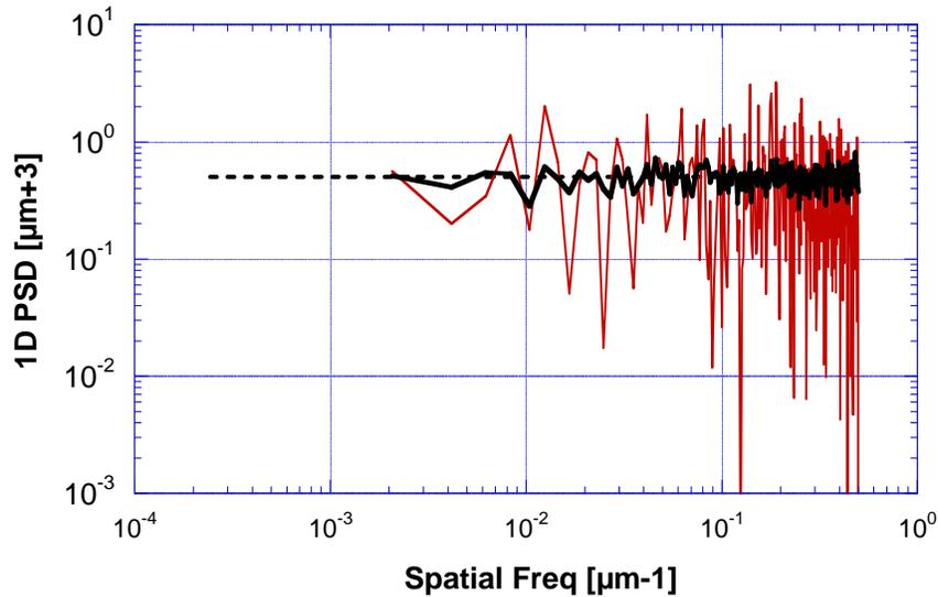
Figure 3: 1D PSD spectrum of the ideal unit-height BPR grating function with 4095 total number of pixels placed on a  $1\ \mu\text{m}$  pitch grid: black (dashed) straight line includes all 4095 points in the calculation; red (solid) irregular line is from a subset of the first 480 points; black (solid) line is average of 9 480-point spectra, each shifted by 400 pixels.
