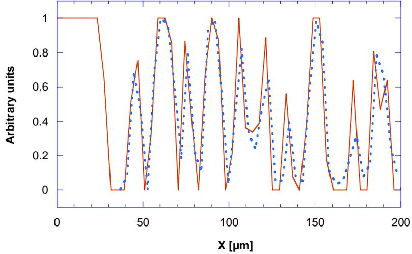
Figure 4: Profile of the first 200  $\mu\text{m}$  of the 4095 element BPR grating with 2.5  $\mu\text{m}$  pitch: ideal computed function resampled to the 3.92  $\mu\text{m}$  grid (red solid curve), and profile measured with the Micromap<sup>TM</sup>-570 microscope with 2.5x objective, (blue dashed curve).
