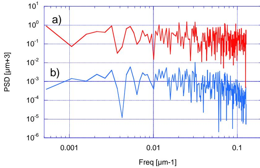
Figure 5: 1D PSD spectrum of the 4095 element, 2.5- $\mu\text{m}$  pitch, BPR grating: a) (red, upper) for the model simulation resampled onto a 3.92  $\mu\text{m}$  grid, and b) (blue, lower) for the profile measured with the Micromap<sup>TM</sup>-570 microscope with 2.5x objective. The simulation and measurement fields of view correspond to the 480 pixel row length in the Micromap. Vertical offset of the lower spectrum is made for clarity.
