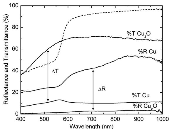
Fig. 1. Transmittance ( $T$ ) and reflectance ( $R$ ) switching behavior as a function of wavelength for a 25-nm-thick Cu film on  $\text{SnO}_2\text{:F}$ -coated glass in 0.1 M NaOH. The dashed line shows the reflectance spectrum of an optically dense Cu film.
