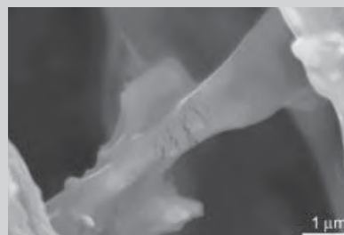
Figure 4. (a) Crack-growth resistance curves for human cortical bone tested in HBSS at 25^\circ\text{C} , with corresponding scanning electron microscopy images of cracks in Young bone at (b) low and (c) higher magnification. The R-curves illustrate that both the initiation toughness (intercept at \Delta a = 0 ) and the growth toughness (slope) are degraded with age.
