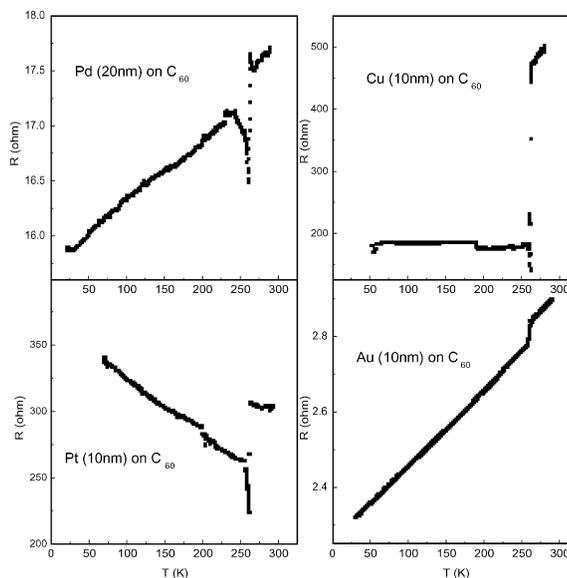
Fig. 3. Resistance vs. temperature behavior for Au, Cu, Pd, and Pt films on  $C_{60}$  crystals.
