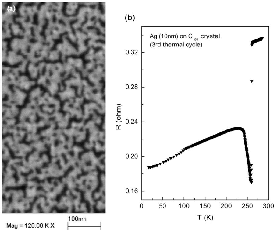
Fig. 1. (a) Scanning electron micrograph of a 10 nm silver film on a  $C_{60}$  crystal. Scale bar is 100 nm. (b) Resistance vs. temperature for a similar film.
