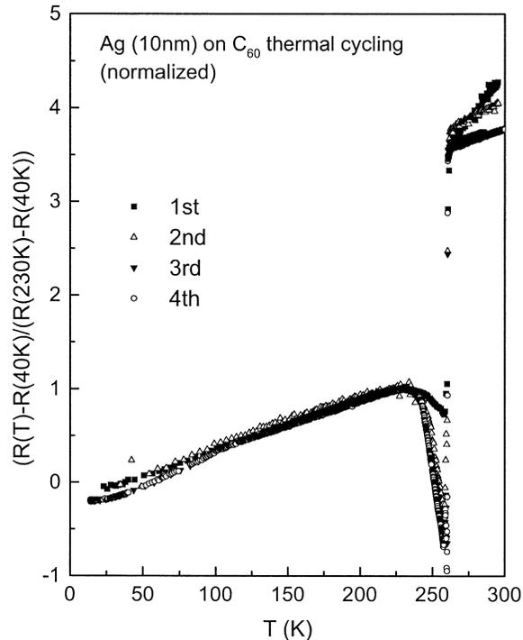
Fig. 4. The data of Fig. 2(a) rescaled according to the strain gauge model.
