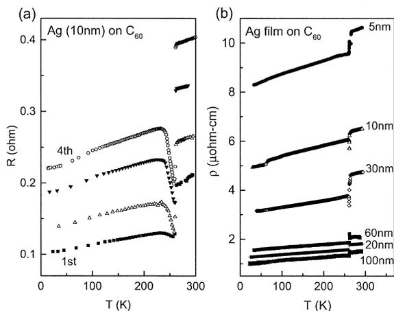
Fig. 2. (a) Resistance behavior of the 10 nm Ag film on  $C_{60}$  with thermal cycling. Only warming curves are shown for clarity. (b) Resistivity vs. temperature of Ag films with different thicknesses on  $C_{60}$  crystals (first thermal cycle).
