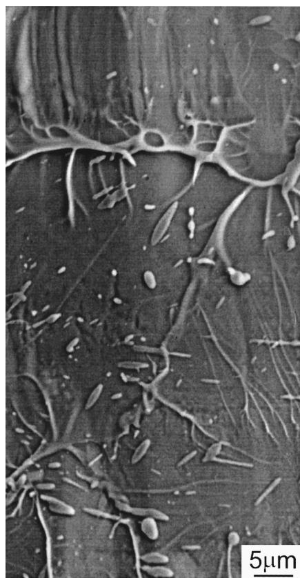
FIG. 4. Scanning electron micrograph of a fracture surface after rupture in nitrogen. Droplets suggestive of local melting are visible. The crack traveled from top to bottom, and the top edge of the micrograph is \sim 10 \mu\text{m} from the root of the notch. Similar features were found on surfaces ruptured in air.
