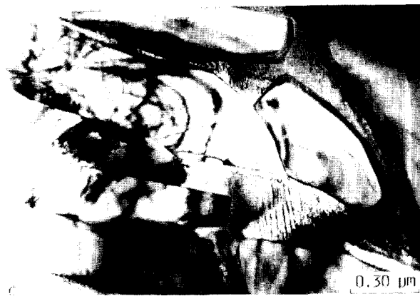
Fig. 6. (a) High-magnification and (b) low magnification bright-field transmission electron micrographs of the growth of Nb 3 Al colonies from grain boundaries, in the hot-pressed and 24 h aged (1800 °C) Nb–6wt.%Al alloy during early stages of the peritectic transformation and (c) in the fully transformed condition. Note the bend contours in the grains and the high density of dislocations in the Nb ss filaments.
