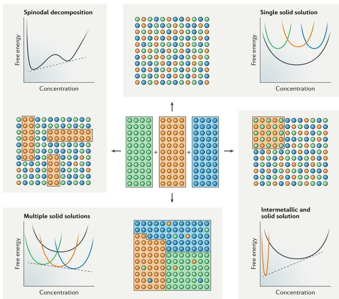
Fig. 1 | **Possible mixing reactions for three alloying elements.** Some of the possible reactions that can occur when three different elements, represented by the red, blue and green spheres, are mixed in equal proportions, including spinodal decomposition, formation of single or multiple solid solutions or precipitation of an intermetallic compound in a solid solution.
