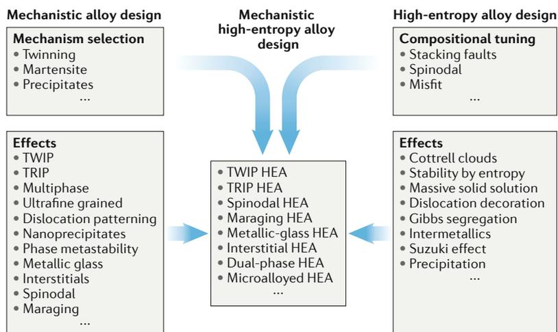
**Fig. 4 | A mechanistic approach to the design of high-entropy alloys.** Established effects from conventional alloys such as twinning-induced plasticity (TWIP) or transformation-induced plasticity (TRIP) can be combined with massive solid solution and its associated degrees of freedom for compositional tuning of stacking-fault energy or desired precipitates for the design of several types of new high-entropy alloy (HEA) classes.
