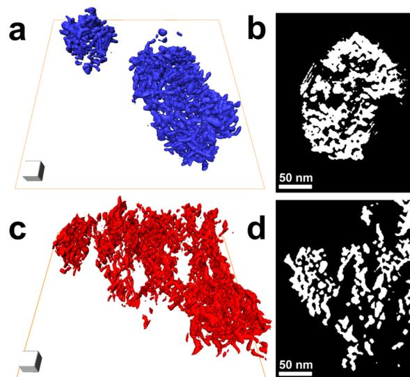
**Figure 3.** Electron tomography reconstructions of tQD-SEBS nanocomposites. (a,c) Perspective image of isosurface reconstruction of compression-sensing and tension-sensing aggregates, respectively, produced by electron tomography. White scale cube has 25 nm sides. (b,d) Thresholded 1.13 nm slices of the tomogram representative of the internal structure of the compression-sensing and tension-sensing aggregates, respectively.
