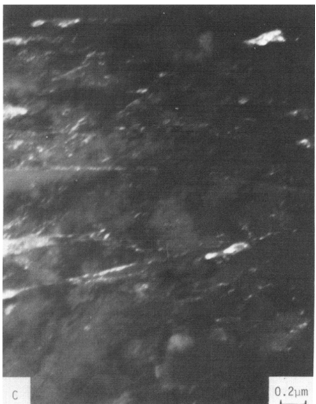
Fig. 20—Transmission electron microscopy of 300-M steel oil quenched and tempered at 400°C. (a) Bright field image revealing martensitic lath structure, (b) dark field image of (200) \gamma reverses contrast of austenite, (c) dark field image of (102) cementite reflection reverses contrast of discontinuous carbide film at lath boundary, (d) diffraction pattern of [\bar{1}11]\gamma || [0\bar{1}0] \text{Fe}_3\text{C} || [011]\alpha zones. A is (200) \gamma , B is (102) \text{Fe}_3\text{C} .
