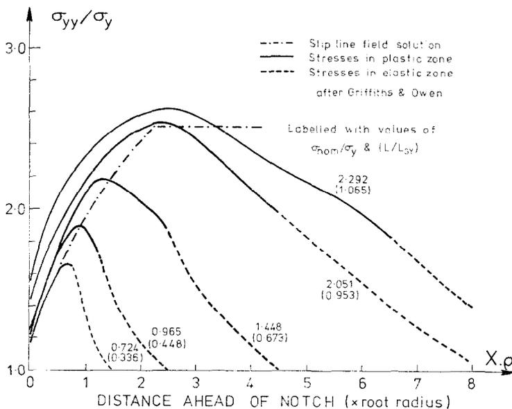
FIG. 9. Distribution of longitudinal stress ( $\sigma_{yy}$ ) acting directly ahead of a rounded notch ( $\theta = 45^\circ$ ) in plane strain at various loads ( $L$ ) from plastic-elastic finite-element solution due to GRIFFITHS and OWEN (1971). For material obeying von Mises' yield criterion with linear work-hardening.
