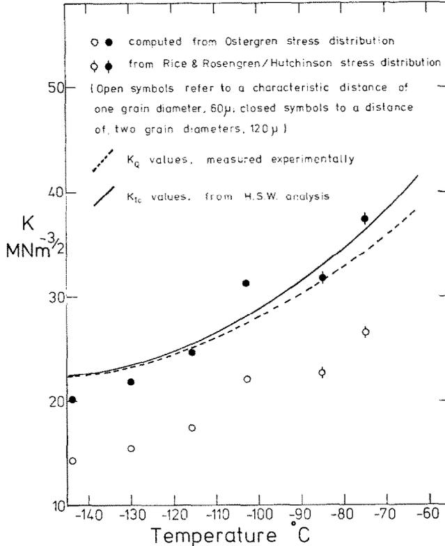
FIG. 7. Comparison of the variation of fracture toughness with temperature between experimental values ( $K_Q$  and  $K_{Ic}$ ) and predicted values for characteristic distances of one and two grain diameters.
