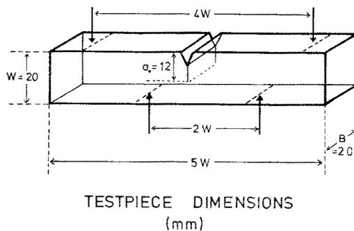
FIG. 2. Geometry of a single edge notched bend test-piece. (Specimens were fatigue pre-cracked to a crack length of 12 mm, i.e.  $a_0/W = 0.60$ .)
