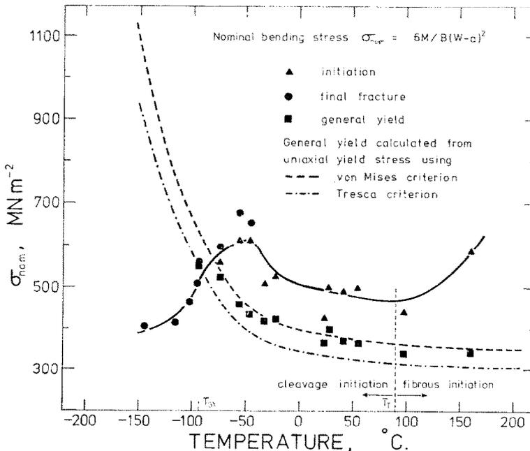
FIG. 4. Experimental general yield and fracture stresses (plotted in terms of nominal bending stress) vs. temperature for pre-cracked bend specimens. Fracture stresses are plotted at initiation and at final failure; these stresses are coincident for temperatures  $\lesssim -90^\circ\text{C}$ .
