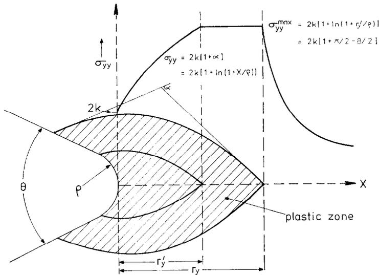
FIG. 1. Schematic longitudinal stress ( $\sigma_{yy}$ ) distribution ahead of a rounded notch, radius  $\rho$ , at general yield; rigid/plastic slip-line field solution. ( $\sigma_y = 2k$ , Tresca criterion, and  $= \sqrt{3}k$ , von Mises criterion.)
