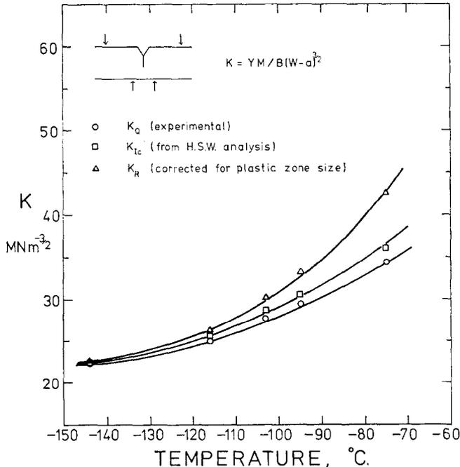
FIG. 5. Variation of critical values of stress intensity at failure. Corrections to experimental values,  $K_Q$ , taken using plastic zone size approximations,  $K_R$ , and analysis due to HEALD, SPINK and WORTHINGTON (1972) (H.S.W.),  $K_{Ic}$ .
