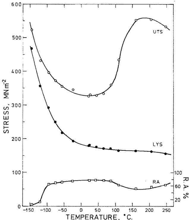
FIG. 3. Variation of uniaxial tensile properties for high-nitrogen mild steel over the temperature range  $-150$  to  $250^{\circ}\text{C}$ . Plotted are the lower yield stress (LYS), the ultimate tensile stress (UTS), and the reduction in area (RA).
