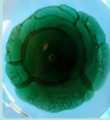
Hydraulic fracture with segments at leading edge created in laboratory [Germanovich et al. 2007]
