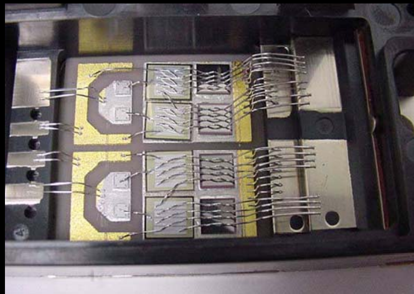
Internal view: 2 80 A SiC MOSFETs and 2 50 A SiC JBS diodes
