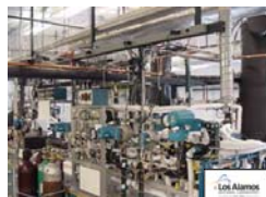
Chemical process development involving engineers, chemists, materials scientists, and computational physicists to build models from lab scale data for process scale-up. Capability for harsh environments (pressure, temperature, acid, base)
