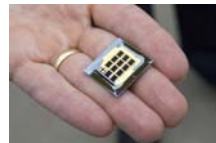
"Black Silicon" Nanocatalytic Wet-Chemical Etch emerged from work by NREL photovoltaic researchers that demonstrated that "black silicon" solar cells, which have been chemically etched to appear black, can better absorb the sun's energy.
