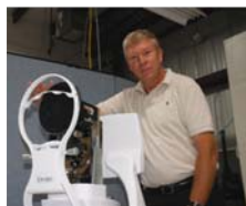
Dan Neal of Wavefront Sciences with iDesign, a wavefront aberrometer providing high-resolution eye measurements to replace five different ophthalmic instruments.
