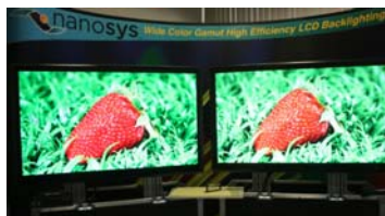
Nanosys quantum dot filter yields richer colors. (Source: Nanosys)
