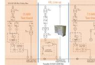
Electrical design enables Utility Scale Hardware-In-the-Loop Testing with turbine under test and grid simulation
