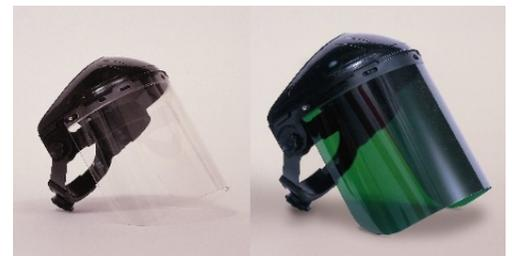
UV-absorbing full face shields should be worn in addition to safety glasses or goggles (goggles may not provide sufficient face protection). Severe skin burns can happen in a very short time, especially under the chin (which is often left exposed).
