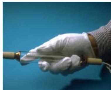
Install the lamp with the proper polarity of electrical wiring. Do not stress the glass parts when tightening electrical connections. Replace the lamp when it reaches its lifetime limit. An old lamp having a darkened glass envelope has a high likelihood of exploding and should be replaced.
