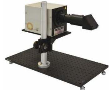
Solar simulators fall into one of three classes: A, B, or C, based on three characteristics: spectral match to sunlight, non-uniformity of the light beam and stability of the light beam over time. If a manufacturer does not clearly specify the class and tolerances for these characteristics, then more likely this is a xenon light source rather than a solar simulator.
