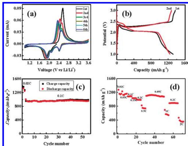
**Figure 4.** (a) CV curve at 0.05 mV s<sup>-1</sup> scanning rate; (b) galvanostatic discharge/charge profiles at 0.02C rate; (c) cycling performance at a constant current rate of 0.1C after initial activation processes at 0.02C for two cycles; (d) reversible capacity vs current density (rate capability). The GO-S nanocomposites were heat treated in Ar environment at 155 °C for 12 h.
