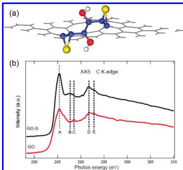
**Figure 3.** (a) Representative pattern of GO immobilizing S. The hydroxyl enhances the binding of S to the C–C bond due to the induced ripples by epoxy or hydroxyl group. Yellow, red, and white balls denote S, O, and H atoms, respectively, while the others are C atoms. Note that the C atoms bonding to S or O are highlighted as blue balls. (b) C K-edge XAS spectra of GO and GO-S nanocomposites after heat treatment in Ar at 155 °C for 12 h.
