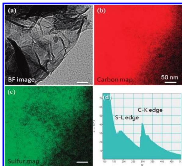
**Figure 2.** TEM bright field (BF) image (a) and the corresponding elemental mapping for carbon (b) and S (c) reveal a homogeneous S coating on the GO flakes. EELS spectrum is shown in (d). The scale bars are 50 nm.
