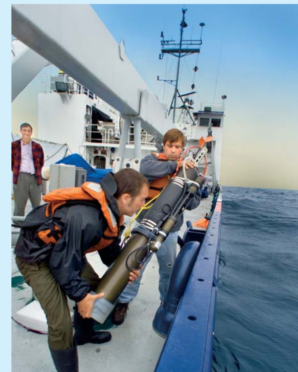
Carbon Explorer floats, called SOLOs, are launched into the sea by Lab researchers to record temperature, salinity, circulation, and carbon biomass concentrations. Such evidence may reveal valuable information about the fate of carbon absorbed and released by the oceans.
