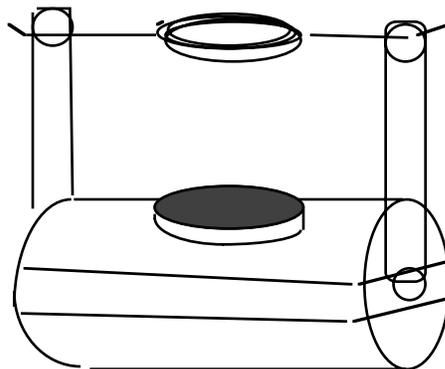
Form supports for your coiled wire by using either duct tape or a thick rubber band to attach the “head” of a safety pin to each end of your “D” size battery.
