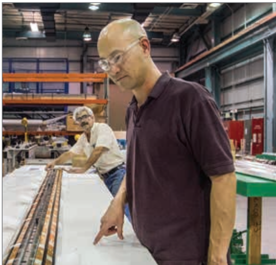
Dan Cheng (foreground) and Ahmet Pekedis fabricate and test a form for a prototype quadrupole magnet for the LHC in Berkeley Lab's superconducting magnet assembly facility.
