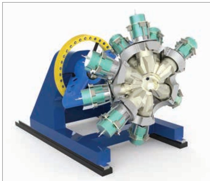
CAD rendering of GRETA, which will support 30 detector modules, giving complete 4- \pi coverage of the volume.
