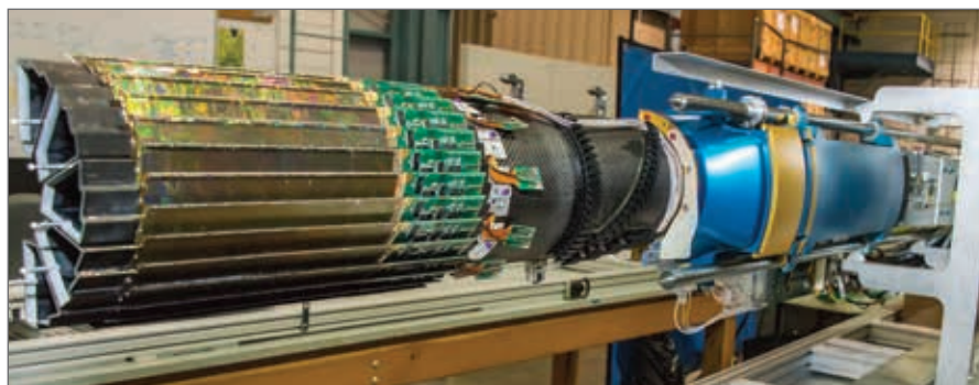
Berkeley Lab led the construction of STAR's Heavy Flavor Tracker. This instrument enables, for the first time, precision tracking measurements of heavy quarks at low momentum.
