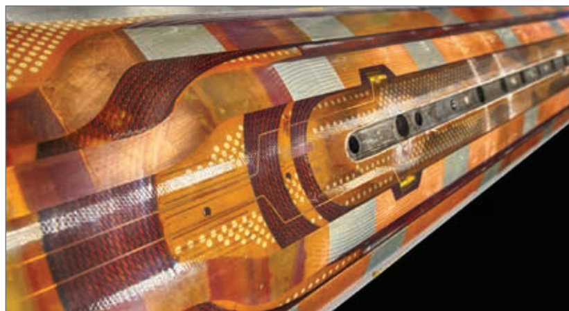
Berkeley Lab partners with Fermi National Accelerator Laboratory (FNAL) and Brookhaven National Laboratory (BNL) on innovative high-field quadrupoles for the HL-LHC project. Photo by Reidar Hahn, FNAL.
