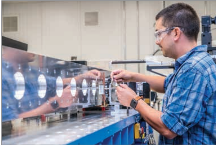
Kyle McCombs in Engineering Division's Undulator Measurement Facility (UMF) measures the magnetic field on a hard X-ray undulator for LCLS-II.
