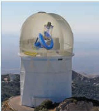
A rendering of the Dark Energy Spectroscopic Instrument (DESI) mounted on the Kitt Peak Mayall telescope. Light from galaxies and quasars will be collected at prime focus by 5,000 robotically positioned fibers and fed to 10 spectrographs.
