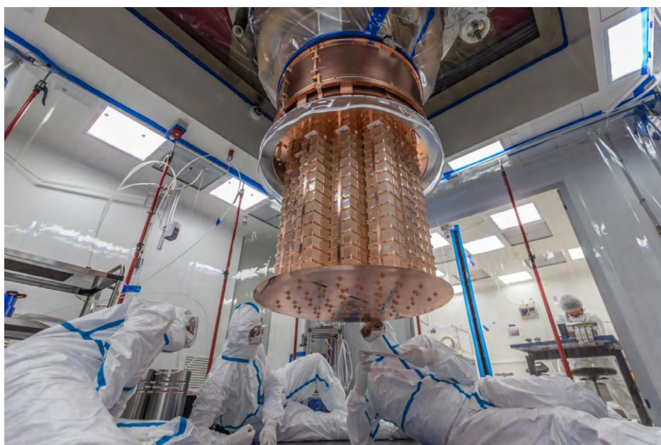
Researchers install tellurium oxide ( \text{TeO}_2 ) crystals in the CUORE experiment at Laboratori Nazionali del Gran Sasso in Italy. These crystals are cooled to below 20 mK during operation. The CUPID experiment will use ^{100}\text{Mo} -enriched lithium molybdate crystals in the same cryogenic infrastructure. Credit: Courtesy of CUORE Collaboration
