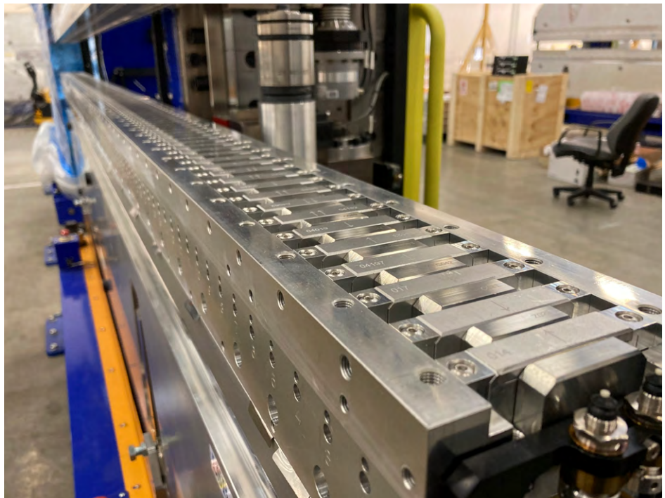
Magnetic arrays on the LCLS-II-HE soft X-ray undulators generate a precise periodic magnetic field that interacts with the electron beam for x-ray production in the LCLS facility.
