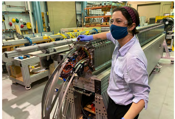
Left, Katherine Ray, a Mechanical Engineer in the Survey & Alignment Group, takes the dimensional measurements of an LHC focusing magnet using the laser tracker system and a hand-held probe. Right, Ray takes the dimensional measurements of an LHC focusing magnet using the laser tracker system and a reflector. Credit: Dan Cheng, Berkeley Lab.
