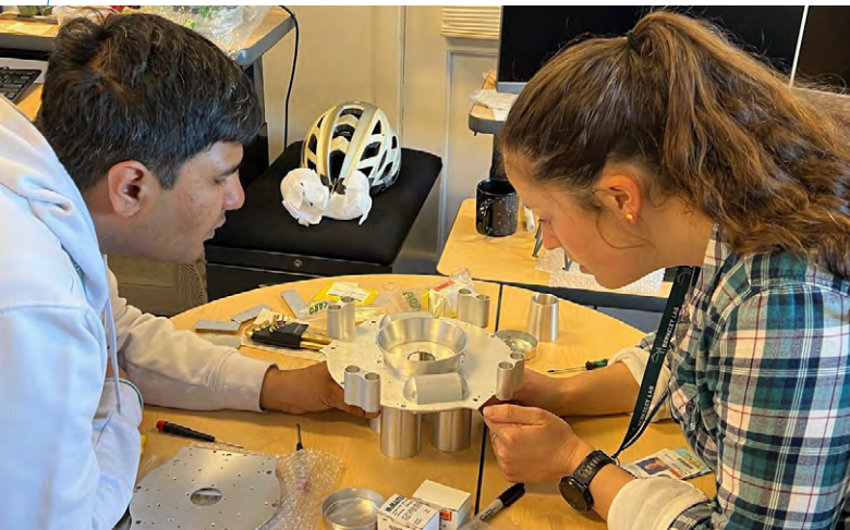
Suvan Ravi (left), a student in UC Berkeley's Undergraduate Research Apprentice Program, and Kaja Rotermund, a Berkeley Lab Physics Division postdoctoral fellow, assemble a scale model of LuSEE-Night payload for an antenna beam characterization test. Credit: Aritoki Suzuki, Berkeley Lab
