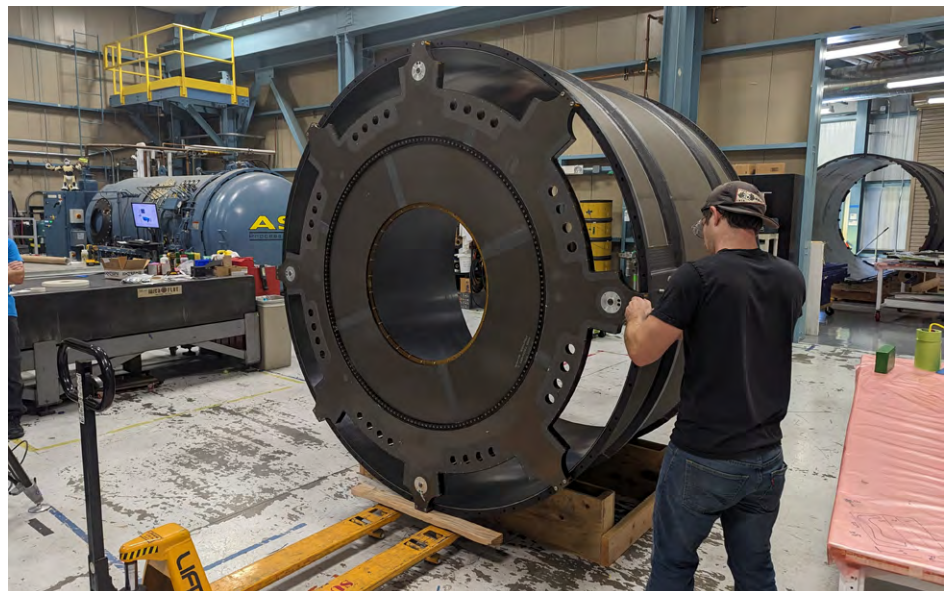
Richard Breese makes adjustments to a structural bulkhead as it is dry fitted to the ATLAS ITk outer cylinder's forward section. Credit: Todd Claybaugh, Berkeley Lab
