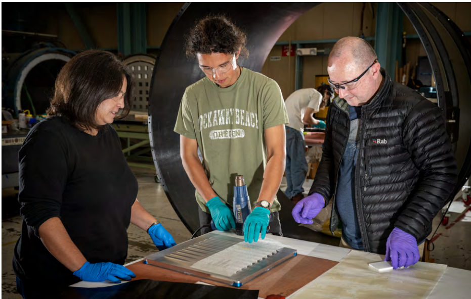
Left to right, Nicole Apadula, a research scientist, Marco McGee Toledo, a mechanical engineer technician, and Eric Anderssen, a staff scientist/engineer, apply a thin layer of coating to one of the corrugated panels that will be installed in the ePIC detector.
