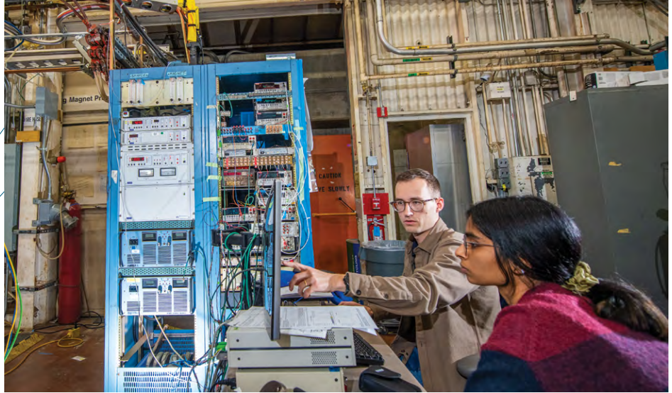
Nandana Menon, a postdoctoral scholar (right), and research scientist Jean-Francois Croteau (left) analyze data for transport current measurements of \text{Nb}_3\text{Sn} wires tested at 4.2 K in a background magnetic field of up to 16-T, for superconducting magnets being built by ATAP's SMP. Credit: Robinson Kuntz, Berkeley Lab
