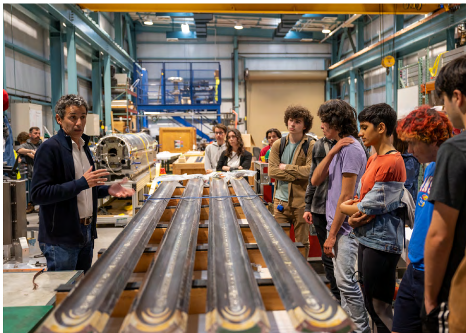
Paolo Ferracin, a senior scientist from the ATAP Division, describes superconducting coils based on niobium-tin superconducting technology for the Large Hadron Collider (LHC) upgrade to Berkeley High School students. Credit: Carl Williams, Berkeley Lab
