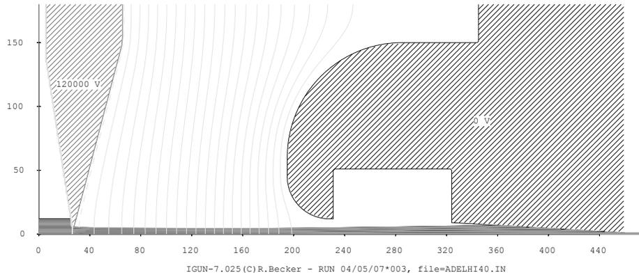
Fig. 2. The ING ion beam extraction and transport simulation. The beam spot size at the target cone is  $\sim 4$  mm in diameter.
