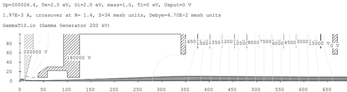
Fig. 4. Ion beam extraction and transport simulation. The ion beam has end energy of 200 keV and the current is ~2 mA. The beam spot size in the end of the simulation is ~9 mm. The length of the simulated area is ~ 150 mm.
