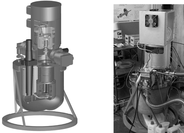
Fig. 5. The first generation axial-type Gamma Tube on its stand. The overall height of the system is 120 cm with the stand, while the ion source/matching-network is 40 cm in height, as well as the high voltage feed-through structure with accelerator column and target. On the right, the Gamma Tube is being tested at LBNL.
