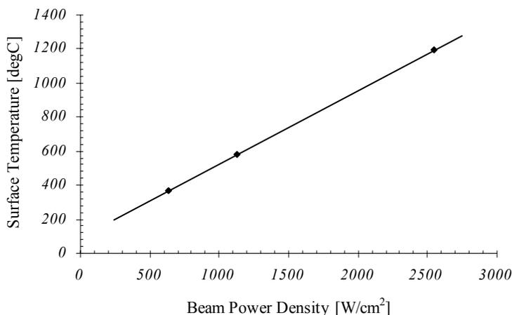
Fig 1. Surface target temperature as a function of beam power density on 0.5 mm titanium layer on copper.
