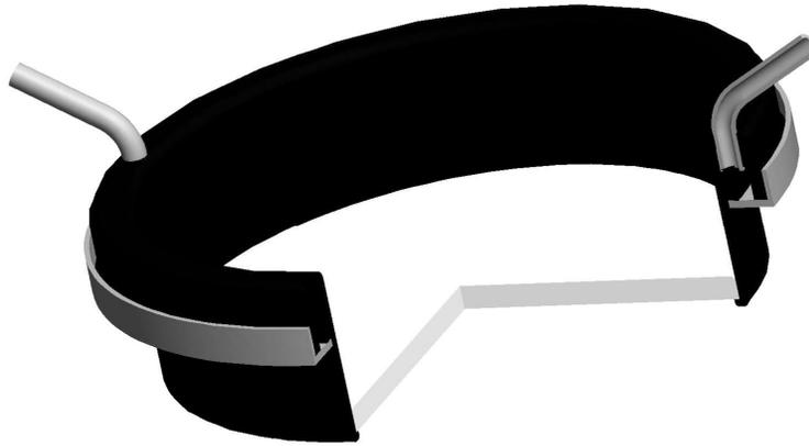
Fig. 6. 3 inch diameter actively water-cooled sapphire RF-window for the PWNG. The window frame is made of copper for low inductive heat and the construction is fully UHV compatible and bakeable to 450 °C.
