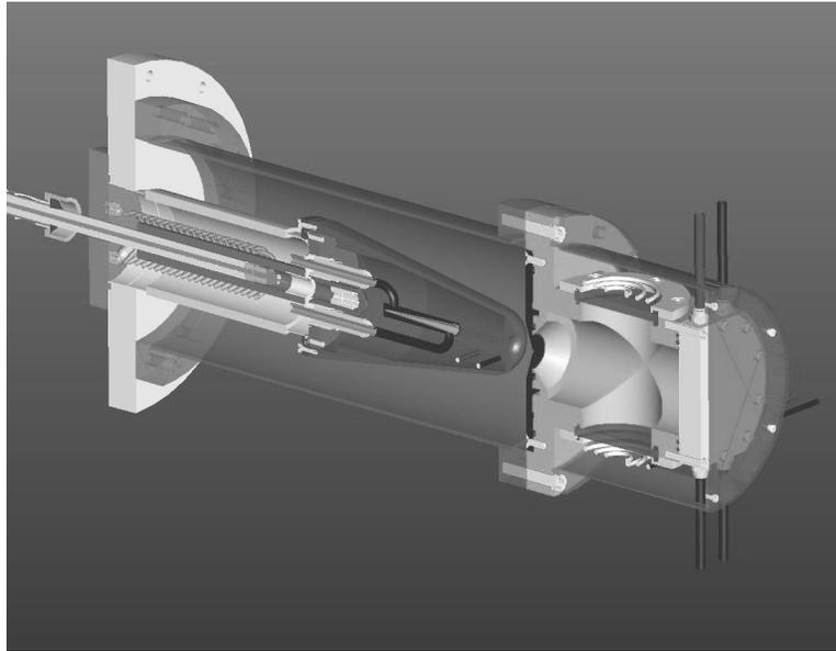
Fig. 3. Imaging Neutron Generator. Note the two-window, actively water-cooled, spiral antenna ion source, cone shape target and high voltage insulator with low resistivity coating.
