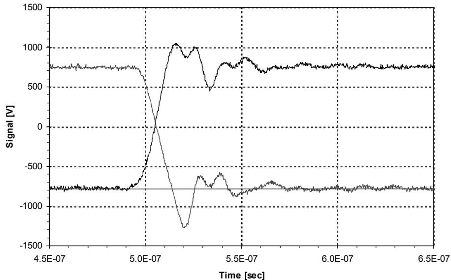
Fig. 7. The fall- and rise-time of the simultaneous voltage pulses of the parallel plates. The measurement is performed by measuring directly the voltage at the plates. A voltage rise- and fall-time of 12 ns is achieved.
