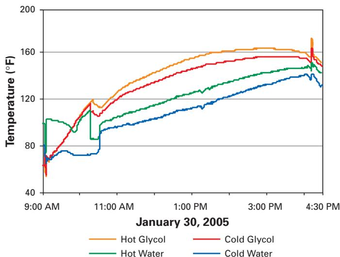
On this particular morning, I was measuring 128°F (53°C) hot glycol entering the heat exchanger and 116°F (47°C) glycol coming back out, but I was only making 102°F (39°C) hot water from the 93°F (34°C) water at the bottom of my tank. I poked around like this for several days and took a few pages of notes. It seemed kind of lousy to me that I was only making 102°F water when I had 128°F glycol coming from the roof.
