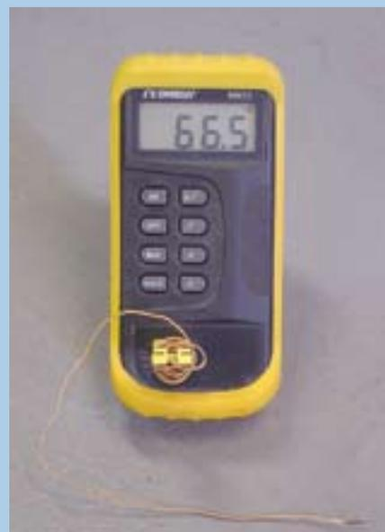
**A simple, handheld temperature meter with a fine-wire, Type K thermocouple is a great tool for quick diagnostics.**
