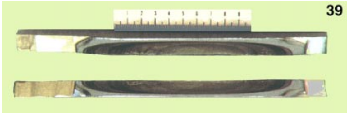
Figure 4. Fracture surfaces from a failed aircraft engine component.
