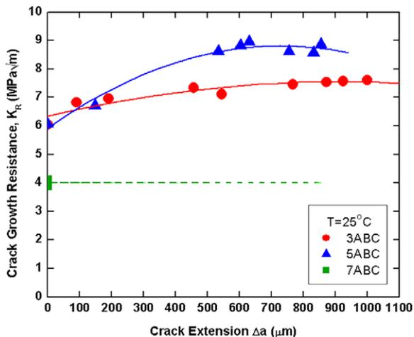
Fig. 3. Crack-growth resistance,  $K_R$ , curves, plotted as a function of crack extension,  $\Delta a$ , for as-hot-pressed xABC-SiC at room temperature.
