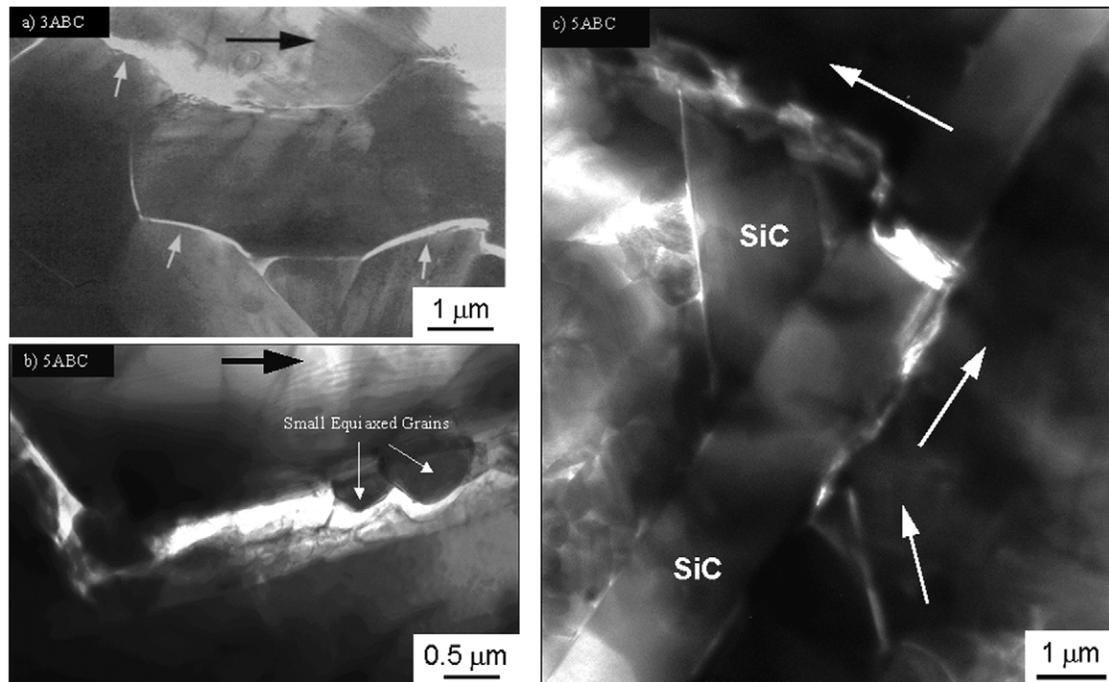
Fig. 7. Transmission electron micrographs near the crack tip in (a) 3ABC, and (b, c) 5ABC grown under cyclic loading at 1300 °C ( $R = 0.1$ ,  $\nu = 25$  Hz). Note in (b) the equiaxed grains also fracture intergranularly and in (c) a failure of an uncracked ligament. Large arrows indicate the general direction of crack propagation, and small arrows point to the primary cracks near the crack tip.
