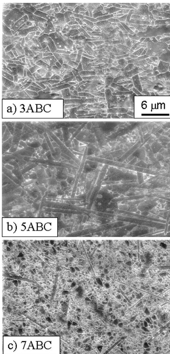
Fig. 1. SEM micrographs of etched surfaces of ABC-silicon carbides showing the characteristic grain structures: (a) uniformly elongated grains in 3ABC, (b) bimodal structure of elongated ( $\alpha$ -SiC) and equiaxed ( $\beta$ -SiC) in 5ABC, and (c) equiaxed grains with sparsely distributed needle-like grains in 7ABC. (Courtesy of Q. Yang).
