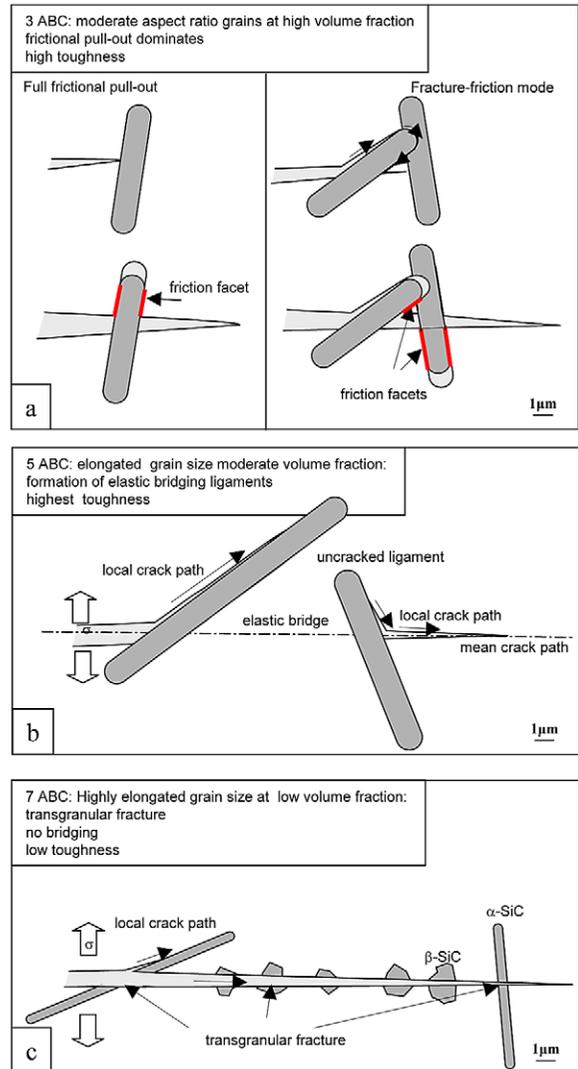
Fig. 9. Schematic illustrations of how the crack paths lead to the development (or not) of crack bridging in (a) 3ABC, (b) 5ABC, and (c) 7ABC-SiC. Note how the predominant mode of bridging in 3ABC is from frictional grain bridging, whereas it results more from uncracked ligaments in 5ABC; in contrast, no bridging is developed in the 7ABC.
