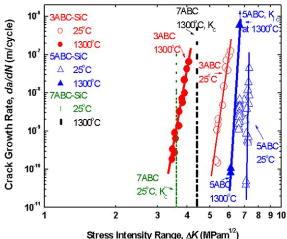
Fig. 4. Cyclic fatigue-crack growth rates,  $da/dN$ , at  $R = 0.1$  in ABC-SiC, as a function of the applied stress-intensity range,  $\Delta K$ , at temperatures of 25 and 1300°C. Note that 7ABC is so brittle that it exhibits no subcritical crack growth, i.e. it fails catastrophically once  $K_{max}$  exceeds  $K_c$ ; the dashed curve for this structure is drawn where  $K_{th,max} = K_c$ .
