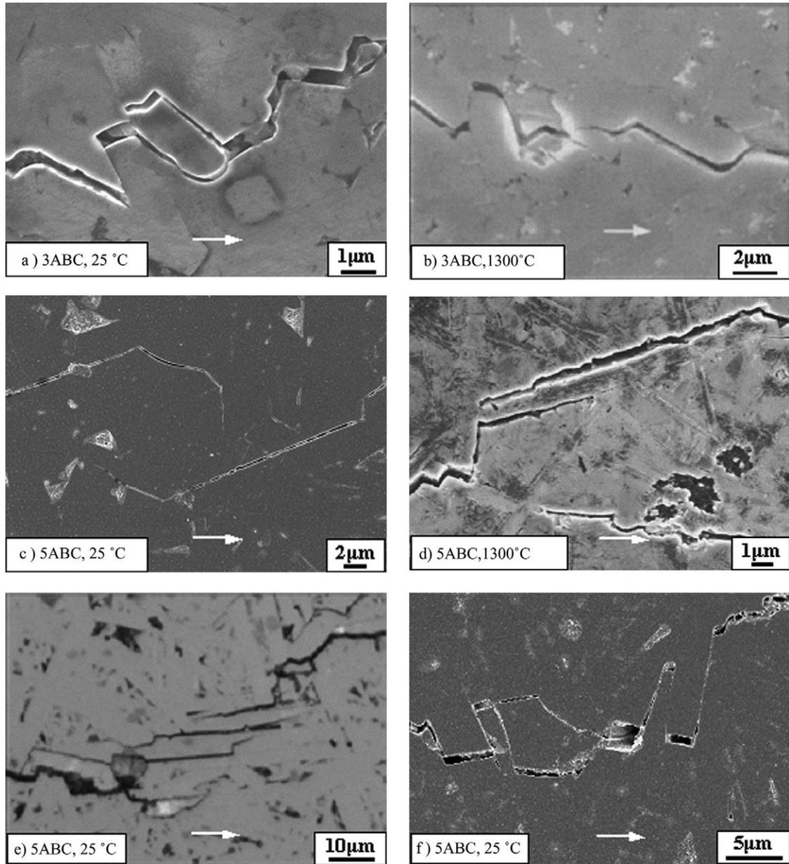
Fig. 6. SEM micrographs of metallographic sections taken perpendicular to the fracture surface showing the crack paths during fatigue-crack growth at 25 and 1300°C for 3ABC (a, b) and 5ABC-SiC (c–f). Frictional bridging (a, b, f) was most common in 3ABC while uncracked-ligament bridges (c, d, e) were predominant in 5ABC. The horizontal arrows indicate the general direction of crack growth.
