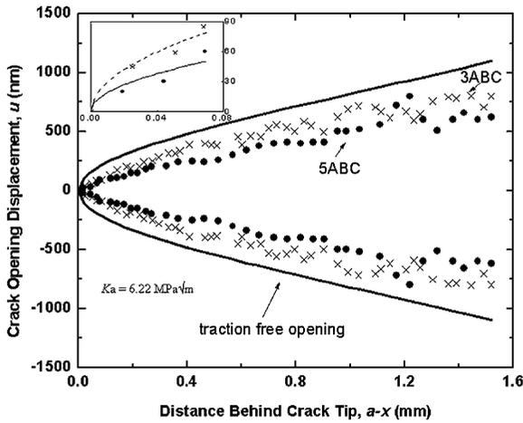
Fig. 8. Comparison of the crack-opening profiles for a monotonically loaded crack in the 3ABC and 5ABC microstructure after R-curve testing. Samples were loaded in situ in a field-emission FESEM to an applied driving force of  $6.2 \text{ MPa m}^{1/2}$ . The inset shows the curve fit for the first  $70 \text{ }\mu\text{m}$  behind the crack tip, where the solid line is for 5ABC ( $K_{tip} = 1.6 \text{ MPa m}^{1/2}$ ), and the broken line for 3ABC ( $K_{tip} = 2.5 \text{ MPa m}^{1/2}$ ).
