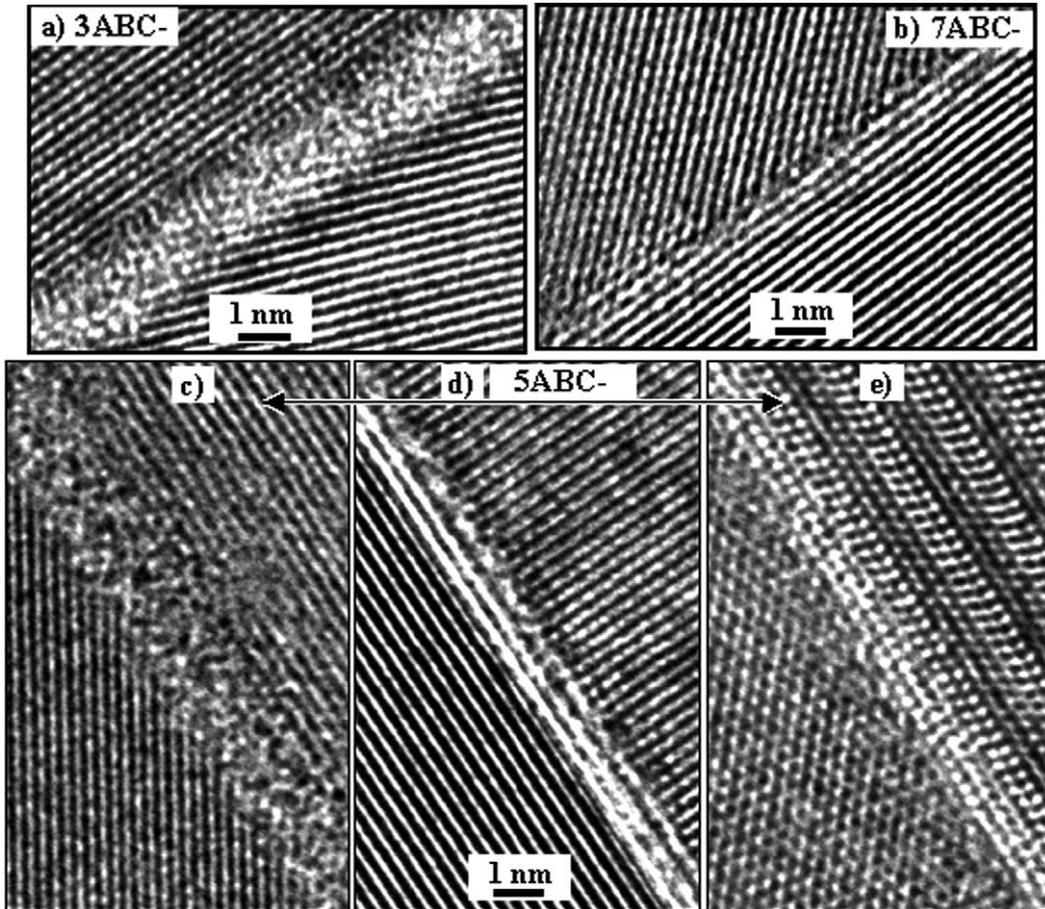
Fig. 2. High-resolution TEM micrographs showing the nature of the grain-boundary films in hot-pressed SiC with different Al content, showing (a) amorphous films in 3ABC, (b) fully crystallized films in 7ABC, and (c) amorphous, (d) partially crystallized and (e) fully crystallized films in 5ABC.
