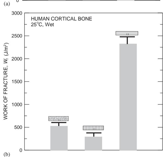
Fig. 5. The measured toughness of bone, in terms of (a) fracture toughness and (b) work of fracture results, obtained in this study for different orientations (schematically shown) with respect to the osteons. The half-error bars indicate one standard deviation; the numbers in (a) are the average toughness values.
