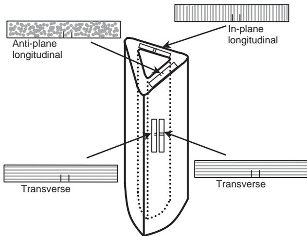
Fig. 1. Schematic illustration of the various specimen orientations, namely transverse, proximal–distal (in-plane longitudinal) and medial–lateral (anti-plane longitudinal), taken from the humeri (with respect to the direction of the osteons, indicated in gray).
