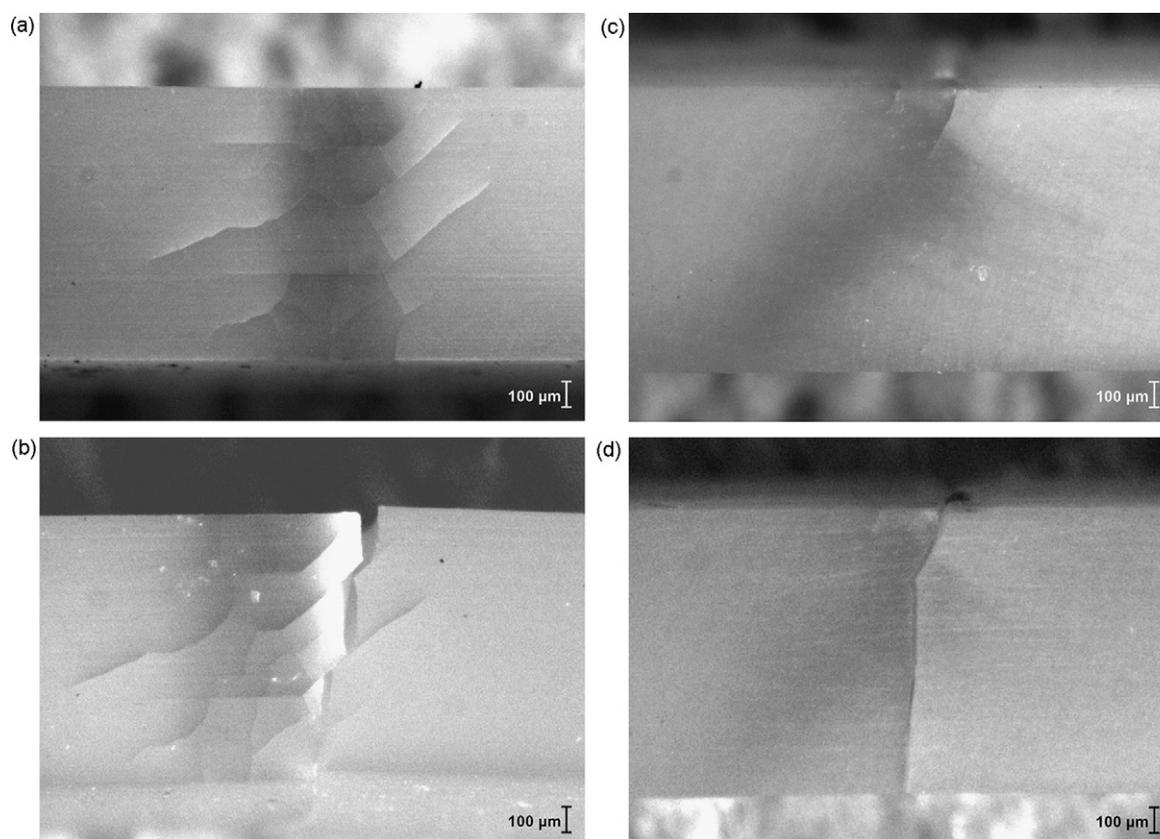
**Fig. 3 – (a) Irradiated surface, group D and (b) same sample, group D, after breaking. The failure is at the site of the initial cracks produced by irradiation. (c) Side view of a sample in group D, showing cracks on top surface and (d) side view of same sample after breaking, showing that the location of failure is a continuation of the initial crack produced by irradiation.**
