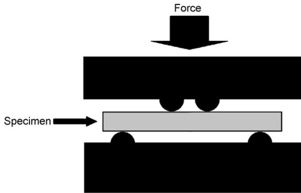
Fig. 1 – Diagram of four-point bending apparatus.
