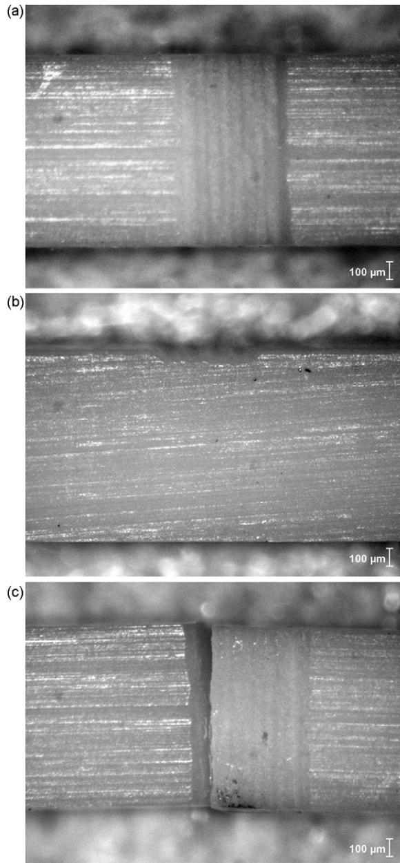
**Fig. 2 – (a) Irradiated surface, group W; (b) side view, group W, showing ablated area at top; (c) same sample from group W after breaking, with failure location at the edge of the irradiated area.**
