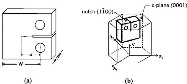
**Figure 1.** Schematic of (a) compact-tension geometry and (b) orientation of crack-plane with respect to crystallographic directions.
