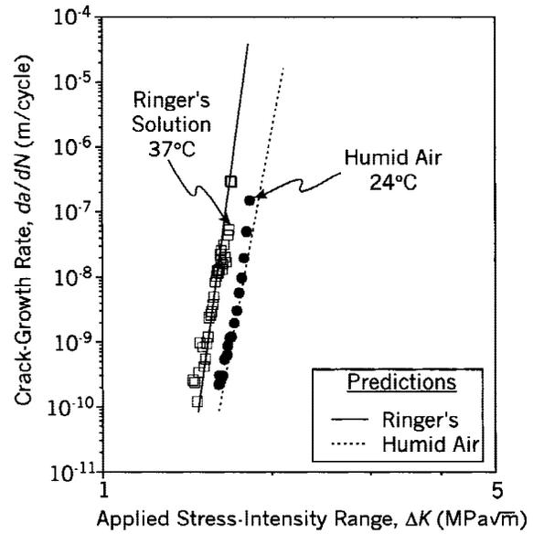
**Figure 3.** Crack growth in sapphire under cyclic loading conditions. Lines represent predictions from the integration of static (fatigue) crack-growth data over the applied loading cycle.
