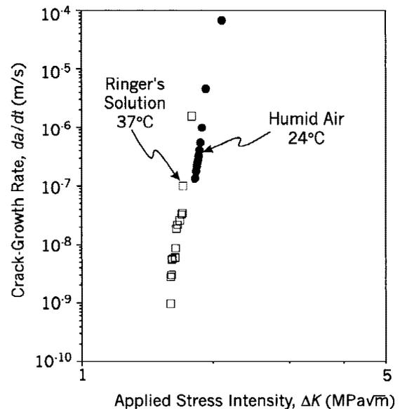
**Figure 2.** Static fatigue-crack growth rates versus applied stress intensity in both air and Ringer's solution.
