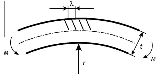
Fig. 1. Bending ductility of bulk metallic glasses. Conner et al. [21,22] have shown that BMG samples below a certain critical thickness,  $t$ , are capable of preventing catastrophic failure by the formation of multiple shear bands. The spacing of the shear bands,  $\lambda$ , decreases with increasing bending moment,  $M$ , and decreasing radius,  $r$ , leading to a more ductile behavior of the BMG.
