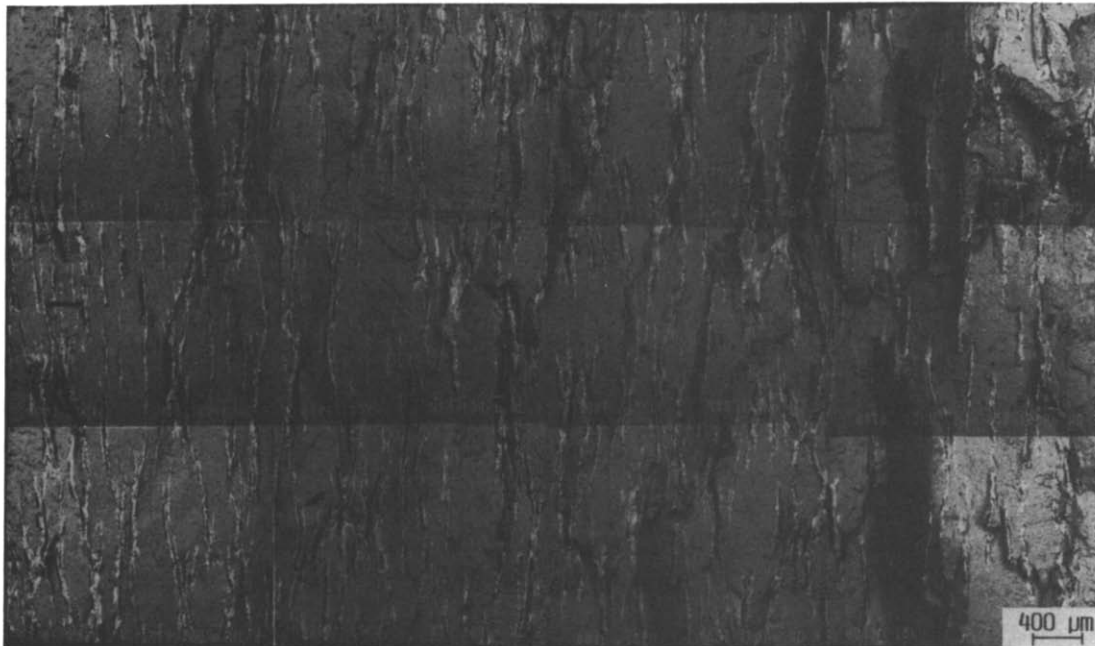
Fig. 3. Montage of SEM micrographs of the fractured surfaces of TiAl + 20 vol.% TiNb composite showing the distribution of ruptured ductile TiNb particles. Note the variations in particle thickness and the non-uniformity of their distribution.
