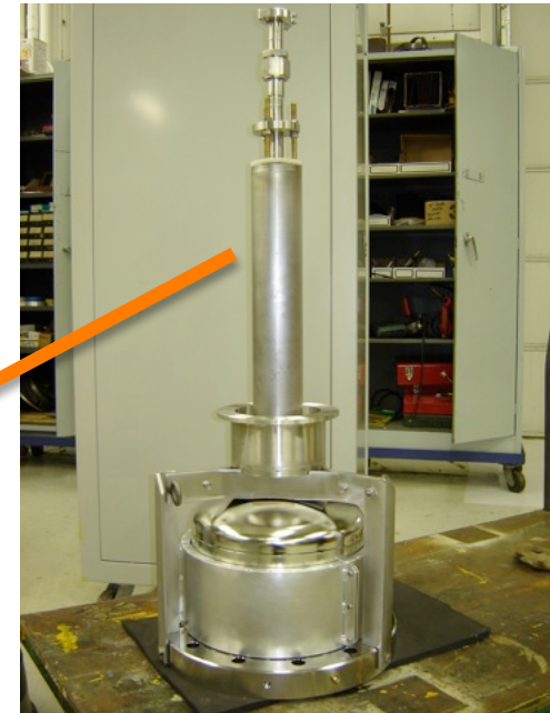
Final electropolished inner vessel top
