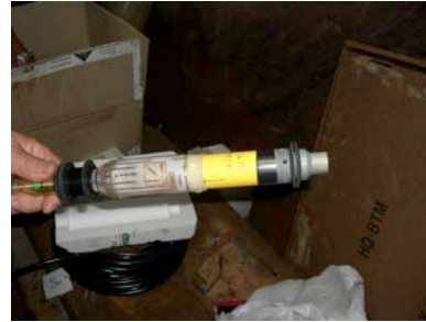
Figure 7: The instrument: Hollow Inclusion Cell with 4 three-element stain rosettes
