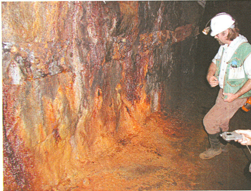
Photo 2. Iron hydroxide precipitates observed in the 21 Ledge ramp approximately 7850 feet below the surface.
