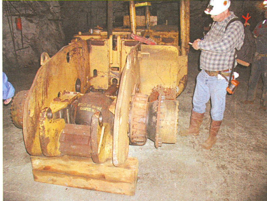
Photo 4. 1700 Level, 7 Ledge LHD shop, 3-yard Wagner LHD chassis abandoned in place.
