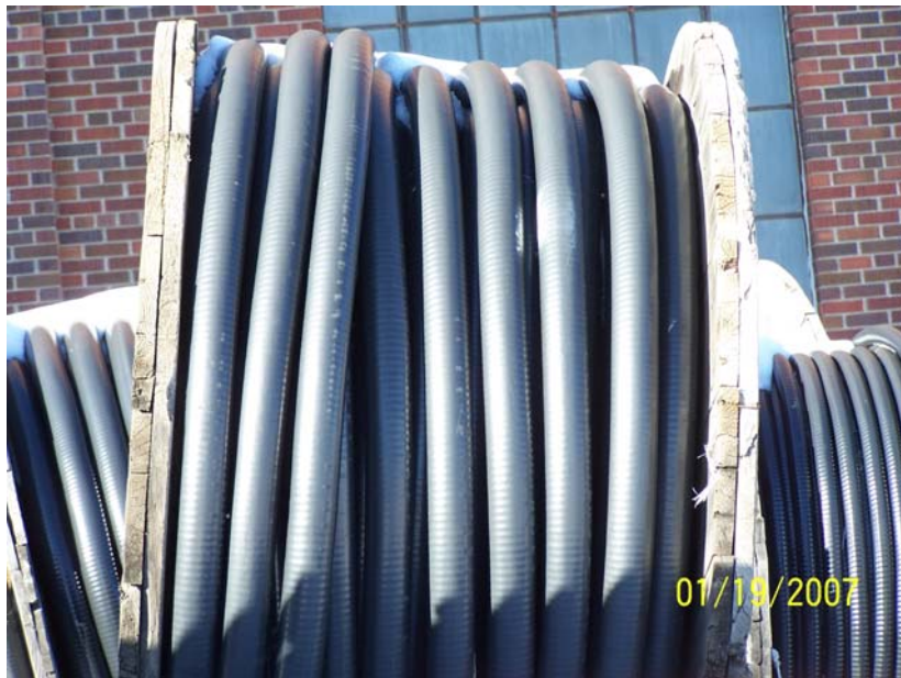
Figure 5.8 – Ross Shaft 5kV Cable
