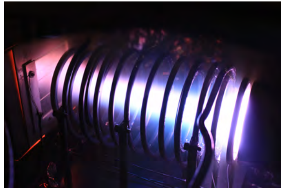
Figure: Photograph of a plasma lens developed for high rate sputter-deposition of oxide films.
