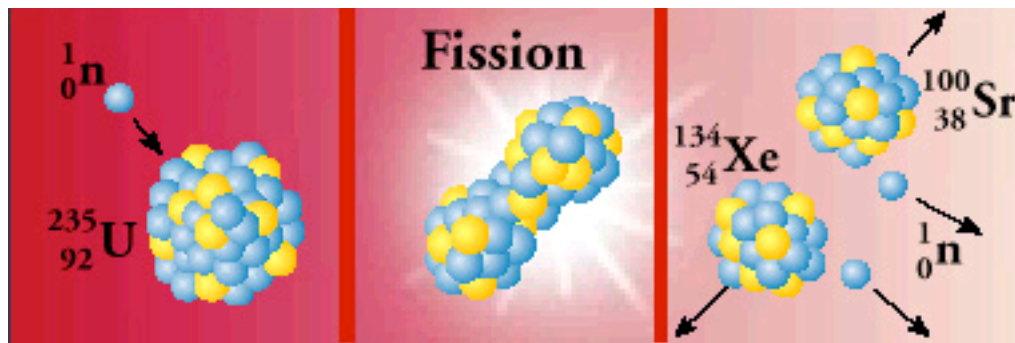
Fig. 14-1. Fission of ^{235}\text{U} after absorption of a thermal neutron.
