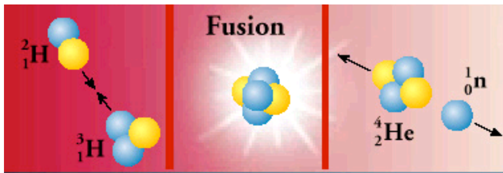
Fig. 14-3. A diagram showing a typical fusion reaction.
