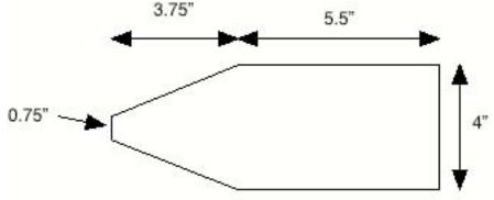
we used had a diameter of 3/4". We used the following dimensions for the scintillators:
