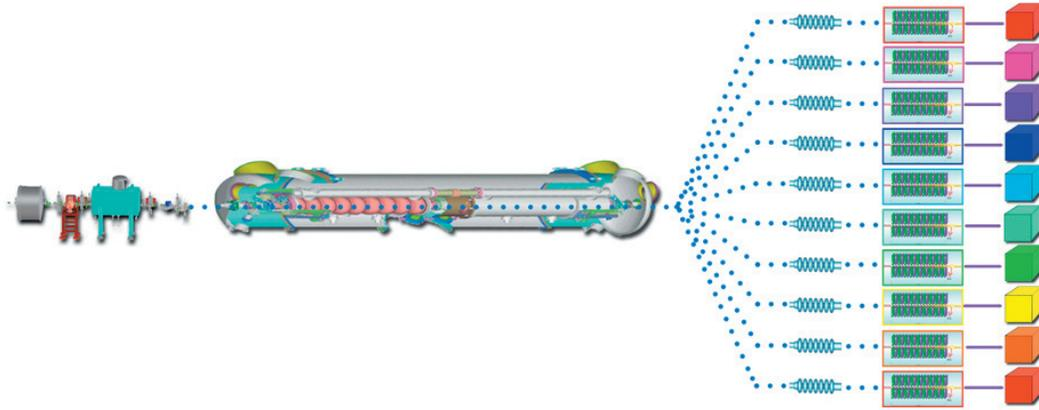
*The next-generation light source facility envisioned for Berkeley Lab would use a superconducting linac to feed 10 or more free electron lasers, each tuned to the user's needs.*
