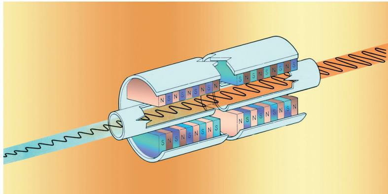
*In a free electron laser, a relativistic beam of electrons is sent through an undulator, an array of dipole magnets with alternating north and south poles. The magnetic field of the undulator forces each bunch of electrons to oscillate back and forth, causing them to emit a laser-like beam of light.*
