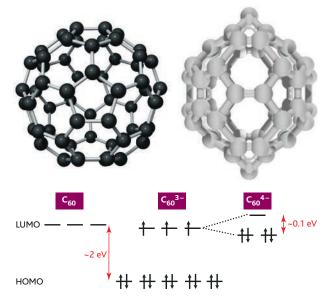
**Squeezed fullerenes.** Geometric and electronic structure of doped  $C_{60}$  molecules. (**Top left**) Undoped and undistorted insulating  $C_{60}$ . (**Top right**) JT distorted  $C_{60}^{4-}$ . (**Center**) The addition of electrons into the threefold degenerate LUMO of  $C_{60}$  and  $C_{60}^{3-}$  and (**center right**) the JT splitting of the LUMO for distorted  $C_{60}^{4-}$ .
